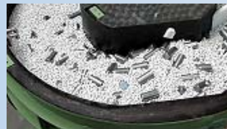
The surfaces of bearing rollers are polished in a rotary vibratory bowl by the Keramo-Finish® process
