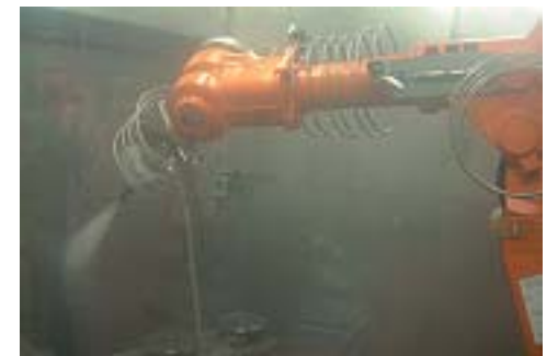
The Rösler high-pressure wet blast system cleans the component at a pressure of 4000 bar
